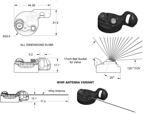
(Antenna chosen based on our discernment; whip increases tire bead clearance and wireless range)
