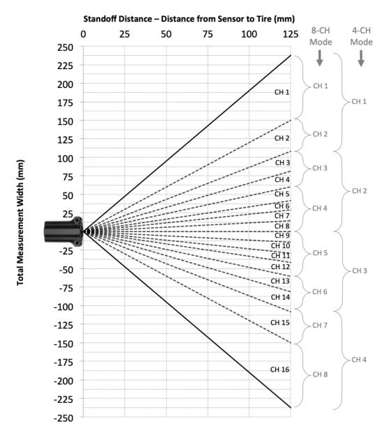
(Angle offset, z-axis rotation, between -5 $^{\circ}$  and +5 $^{\circ}$ , mounts should allow adjustment accordingly)
