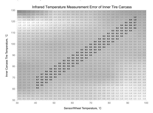
Test Conditions: 1.0 – 3.5 bar, air, 20-50% humidity, infrared channels 5 to 12
