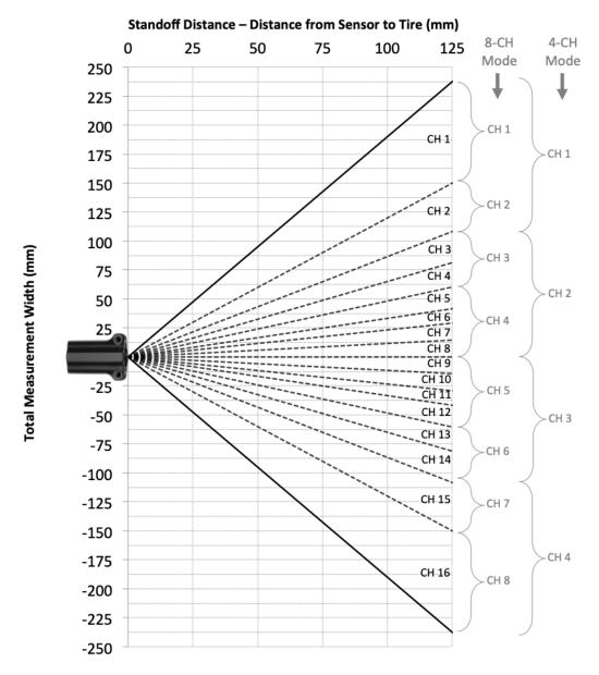
(Angle offset, z-axis rotation, between -5° and +5°, mounts should allow adjustment accordingly)
